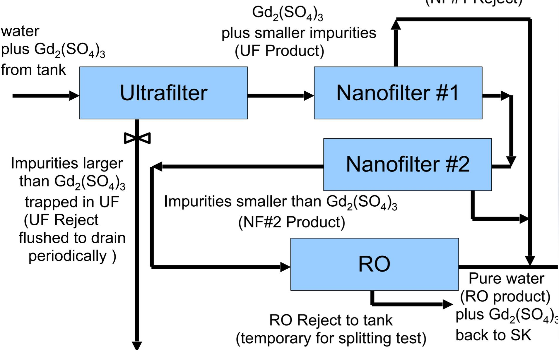
Scaled up design for SK sized tank
